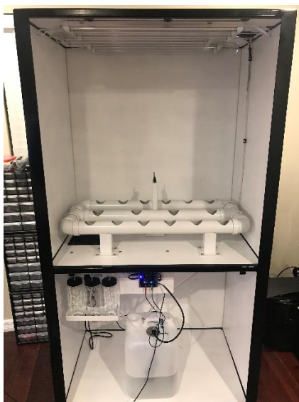
Figure 2: 2 Segment Enclosure Design
